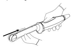
4. Inspect the sheath to ensure there are no holes or tears.
