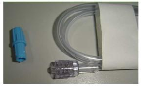
3. Push back the locking nut to extend the connector, as shown in the following figure. The connector should be connected to the transducer's injection/drainage port.
