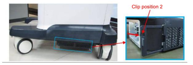
There are 6 dust filters – 2 are located on the left hand side of the system, 2 are located on the right hand side of the system and 2 are located at the front of the system.
